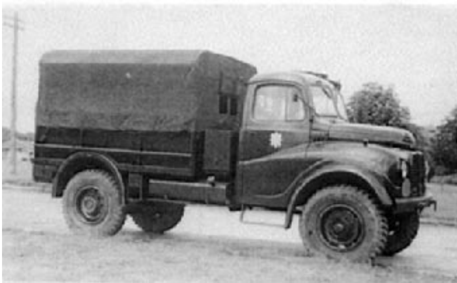
Classic form of the 'K9'. This is an FV 16001 'Cargo' designed to carry a section of soldiers and their kit. As the years went by they got various adornments to suit them for a wide variety of roles in many different arenas.
