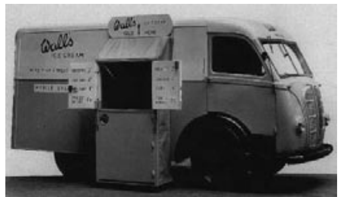
The K8 was Austin's 25 cwt 'commercial'. It was innovative, with doors on either side and at the back, and lively. Walls capitalized on the former features by devising an ingenious sales point the main points of which were later adopted for the much larger coach-based sales and information vehicle.
