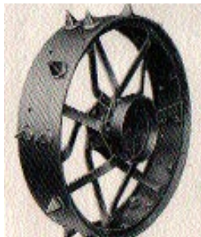
Features included clockwise from top left, a dust sealed Zenith carburettor, a sludge trap in the crankcase that could be opened by using the starting handle to allow sediment to drain out, and a variety of standard accessories such as wheels to suit differing terrains. This is the version with 'spuds' for additional grip.
